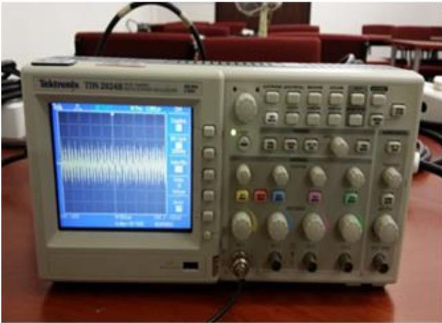
Figure 3: Tektronix TDS2024B DSO used for time domain measurements
