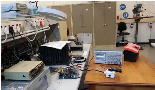
Figure 13: Time domain noise measurement set up in an electronic workshop
