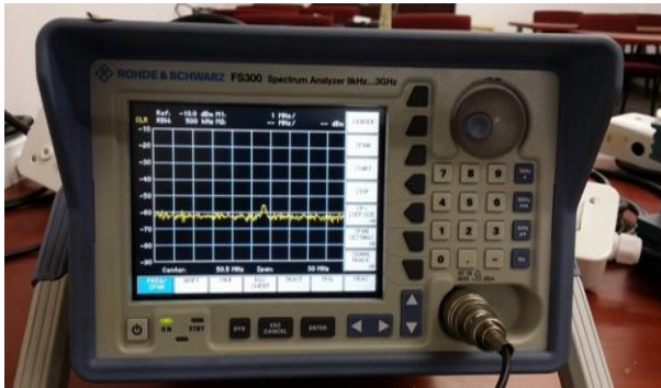
Figure 1: The R&S®FS300 equipment in a set up for background noise measurement in the PLC Laboratory
