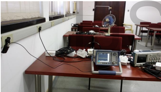
Figure 12: Frequency domain noise measurement set up in the PLC laboratory
